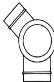
REDUCING 135° STRAIGHT CROSS When Ordering, List: A, B, C, D L = Larger of C or D, + 2"
